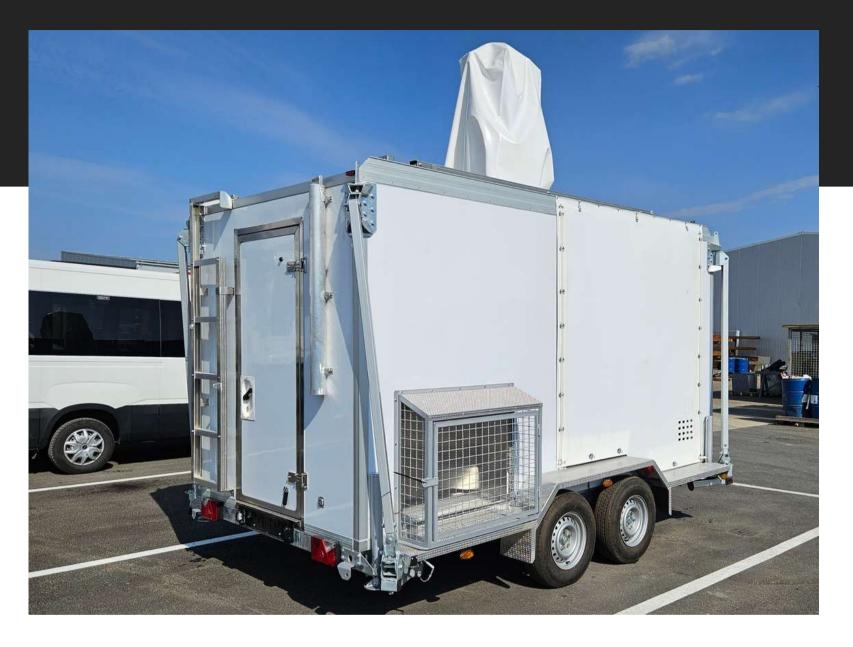
The superstructure is made of insulated composite sandwich panels.
